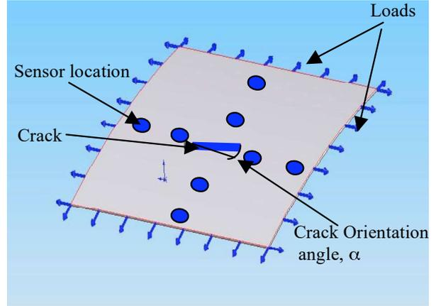
Figure 1. Typical fuselage panel loading.
