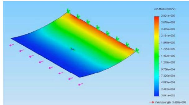
Figure 2. FE model of curved panel with transverse crack.
