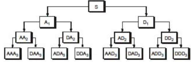
Figure 2. Wavelet packet decomposition [11]; signal s is decomposed as  $s = A1 + AAD3 + DAD3 + ADD3 + DDD3$  at level 3.
