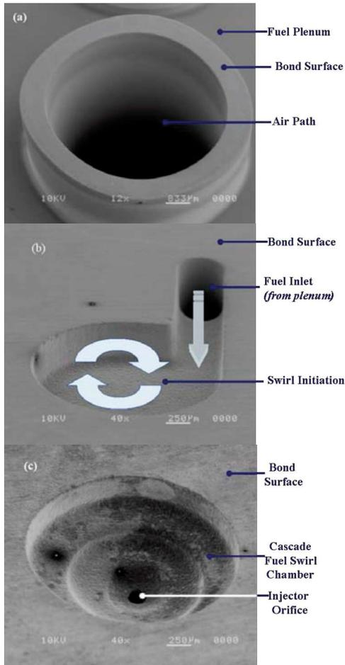
Figure 8. SEM images of SiC substrates which comprise a) fuel plenum, b) fuel inlet that feeds the fuel swirl chamber and c) the fuel swirl chamber with the injector orifice.
