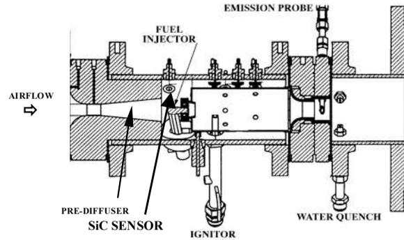
Figure 4. Test rig designed to replicate real instability at engine conditions. Location of the SiC pressure sensor relative to the combustion chamber is shown.
