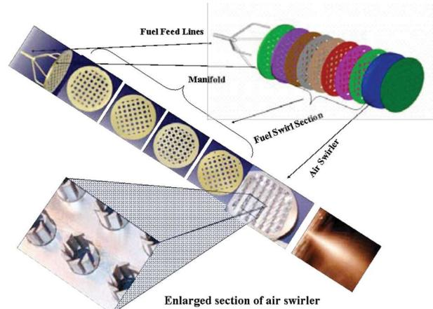
Figure 10. Isometric view of the conceptual model showing the SiC stack (top right), the corresponding fabricated substrates with their various functions (middle), and the magnified air swirler chamber (bottom left).
