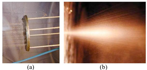
Figure 11. a) Completed SiC MEMS MP-LDI array shows uniform spray pattern, and, b) atomized spray pattern after mixing.
