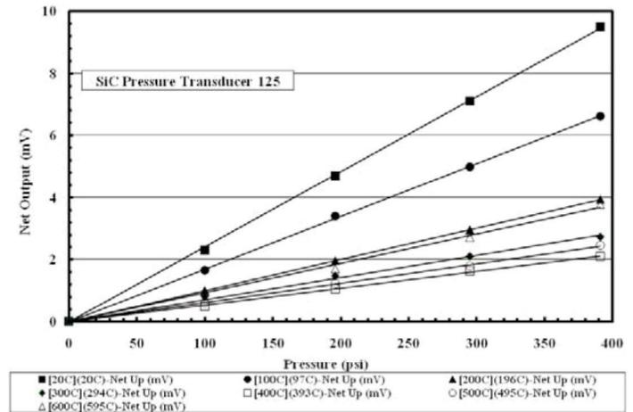
Figure 2. Full-scale net output at 400 psi of 4H-SiC pressure transducer as function of temperature.
