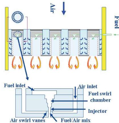
Figure 7. Cross section drawing of the SiC MP-LDI showing air and fuel swirlers and injector sections. Notice the interaction between fuel and air occurs only at the mixing stage inside the air swirl chamber, just prior to burn.
