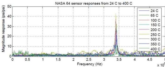
Figure 3. Frequency response of SiC pressure transducer as function of temperature during shock tube test [4].
