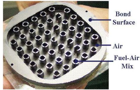
Figure 9. Optical image of the air swirl chamber where fuel and air would mix to induce fuel break up into smaller particle diameters.
