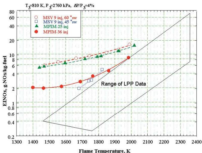
Figure 6. Comparison of flame-tube NO<sub>x</sub> emission from metal MP LDI configurations from 9 to 36 injector array. It shows significant NO<sub>x</sub> reduction with increasing injector array [7].
