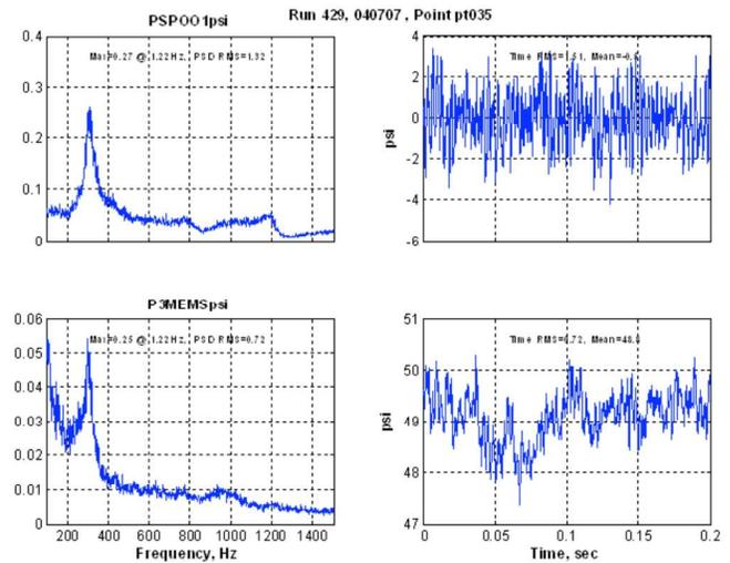
Figure 5. Amplitude spectral density (left column) and brief time history (right column) for the commercial piezoelectric pressure transducer (PSP001) and the SiC pressure transducer (P3MEMS) show the detection of thermo-acoustic instability at 310 Hz by both devices.
