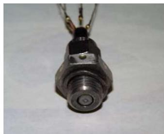
Figure 1. Fully packaged SiC pressure transducer fitted into National Pipe Thread housing rated to operate at 600 °C.
