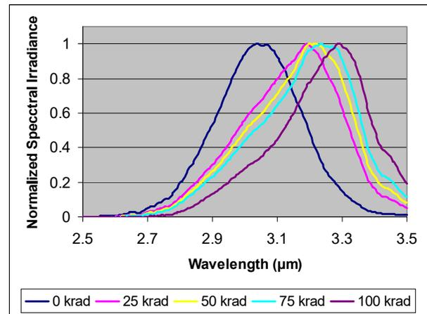
Figure 7: LED 3.4 spectral irradiance vs. metered dose.
