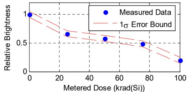
Figure 8. LED 3.4 relative brightness vs. metered dose.
