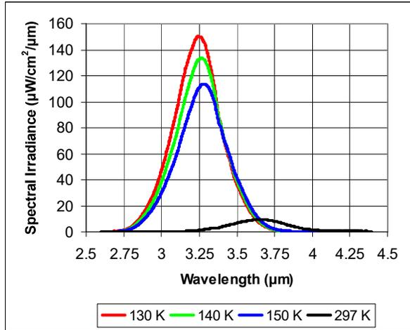
Figure 1. Absolute spectral irradiance as a function of operating temperature for LED 3.6 at a distance of 92 mm.
