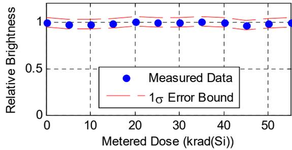
Figure 12. LED 3.8 relative brightness vs. metered dose.
