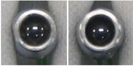
Figure 5. LED with lens before (left) and after (right) more than 10 cryogenic thermal cycles showing no lens damage.
