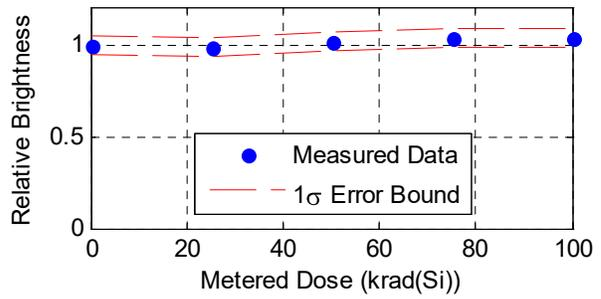
Figure 11. LED 3.6 relative brightness vs. metered dose.
