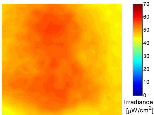
Figure 2. Spatial irradiance map over  $5 \times 5$  deg FOV for lensed LED 3.6 at 92 mm distance operating at 130 K.
