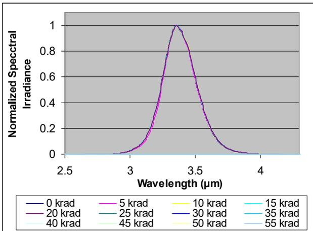
Figure 10. LED 3.8 spectral irradiance vs. metered dose.
