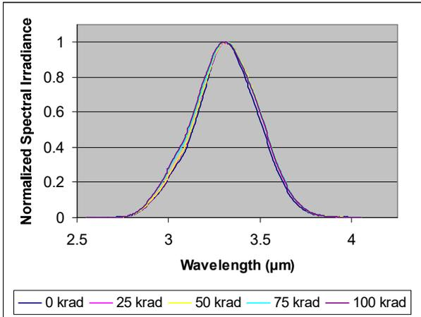
Figure 9. LED 3.6 spectral irradiance vs. metered dose.
