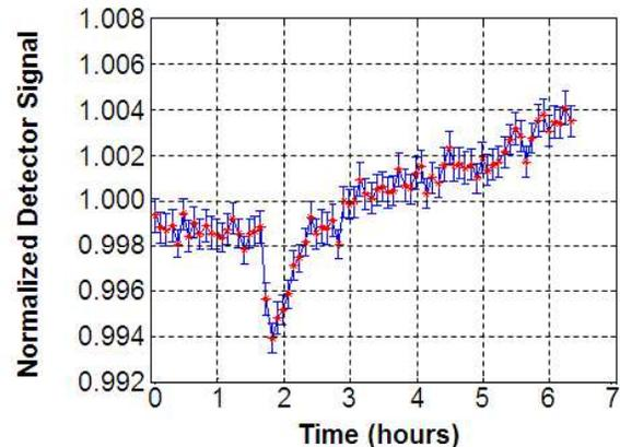
Figure 4. LED stability over 6 hours of operation at constant 130 K temperature.
