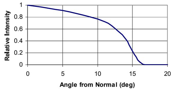
Figure 3. Typical intensity vs. exitance angle at 130 K.
