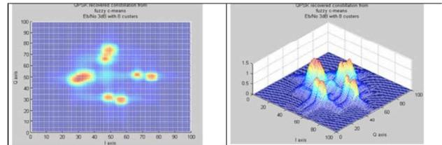
Figure 7. Simulated Fuzzy C-Means Reconstructed Constellation (QPSK 3dB Eb/No).
