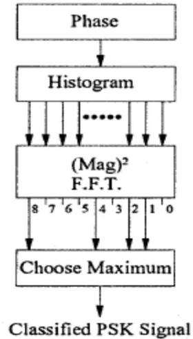
Figure 1. DFT/Phase-Histogram Processing Flow.
