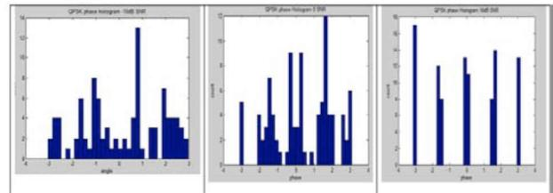
Figure 3. Phase Histogram for QPSK Signal for various SNR.
