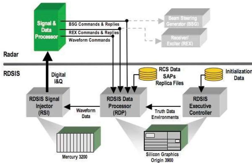
Figure 4. Radar Digital Signal Injection System.
