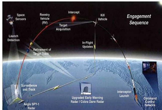
Figure 1. Elements of the Ballistic Missile Defense System.
