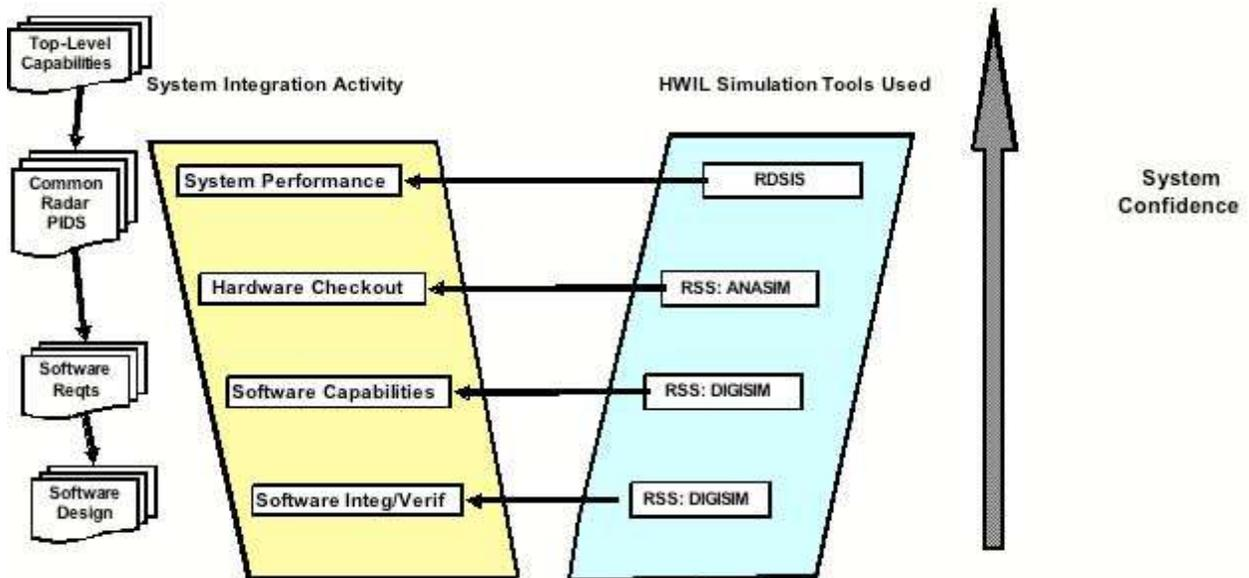
Figure 3. Lifecycle for testing a radar software from requirements to simulation.
