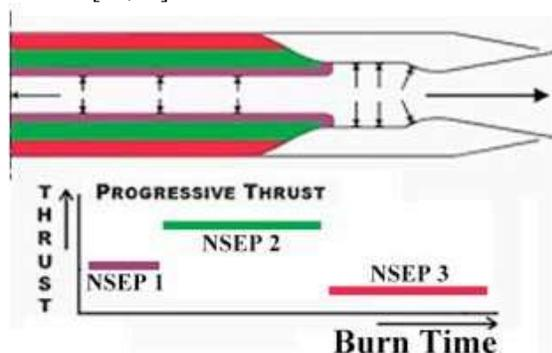
Figure 9. NSEP based thrust profiling in propellant grain through multi-layering of NSEPs with different performance properties ( $I_{sp}$  and Burn Rate).
