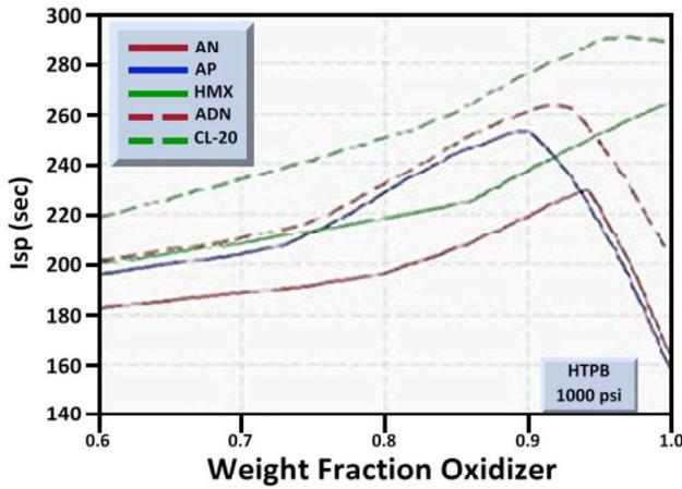
Figure 2. Specific Impulse ( $I_{sp}$ ) as a function of weight fraction of various oxidizers.
