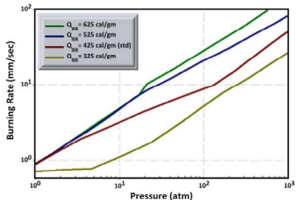
Figure 6. Hermance Model Predicted NSEP Burn Rates based on reaction Q value ( $Q_{RR}$ ) of formulation.
