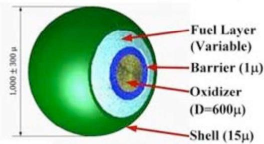
Figure 7. The NSEP (NanoStructured Energetic Particle).
