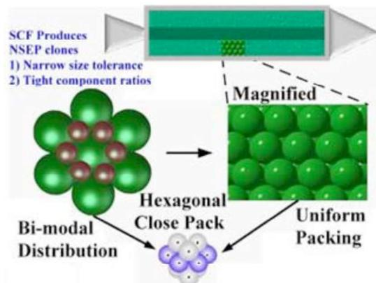
Figure 8. Packing of bi-modal NSEP particle distribution in solid propellant grain prior to binder infusion and casting.
