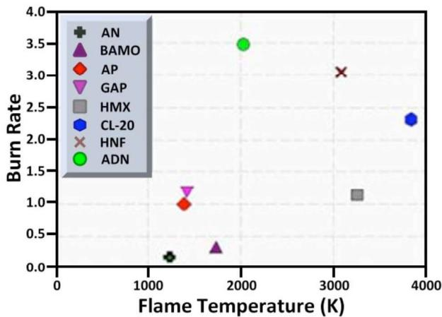
Figure 3. Relative Burn Rates of various potential and current oxidative solid propellant ingredients.
