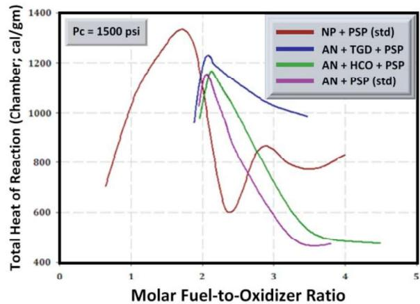
Figure 5. NSEP formulations vs. Standard composition.  $P_c$  is chamber pressure in this figure.
