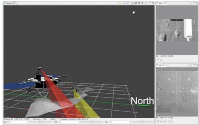
Figure 5. The 3D viewer together with simulated RAC and SSI camera view UI elements. The 3D viewer is displaying RAC and left SSI camera view frustums as well as a glyph (upper right) indicating the location of the sun.
