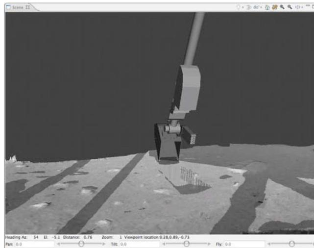
Figure 2. The Mercator interactive 3D viewer with time of day shadows enabled and a simulated trench shown.
