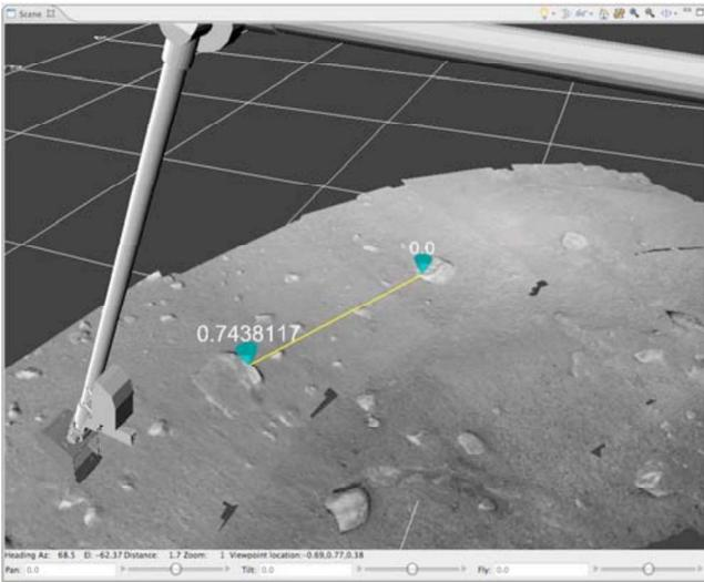
Figure 3. The distance measurement tool in the 3D viewer. The end markers of the tool follow the surface and can be directly positioned with mouse and cursor.
