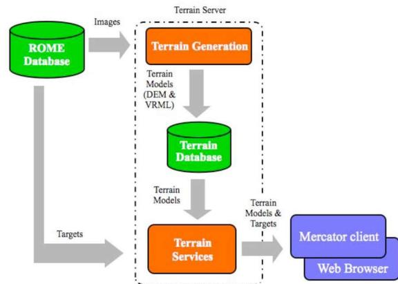
Figure 9. Overview of ARC 3D visualization data flow.
