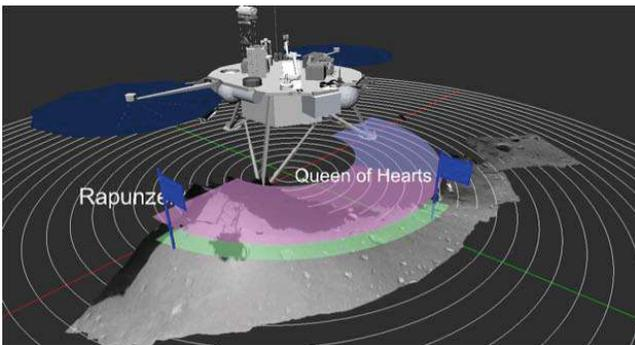
Figure 4. The 3D viewer showing named science targets, reachability map overlay, and polar grid.
