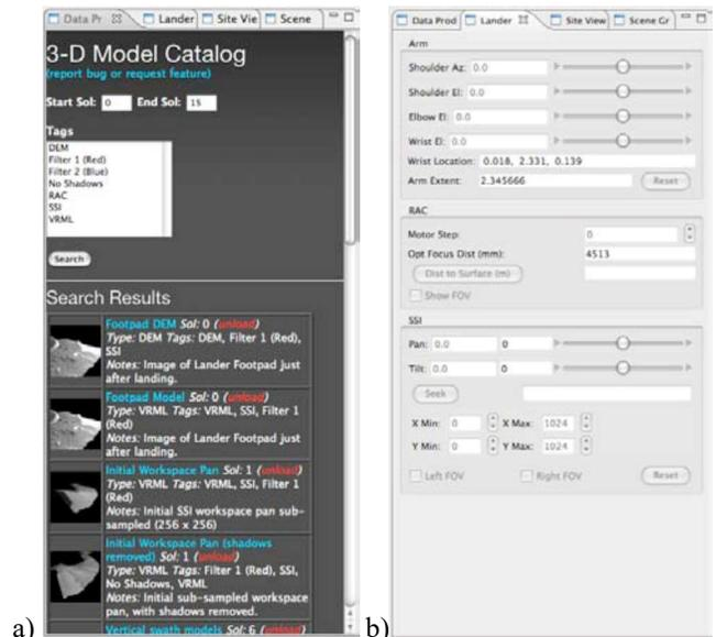
Figure 6. Mercator tabbed UI element. a) terrain model browser panel, b) lander control panel.
