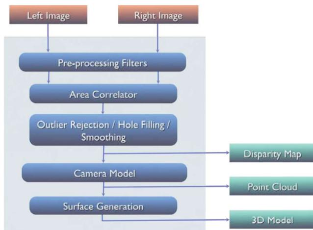
Figure 7. Ames Stereo Pipeline data flow diagram.
