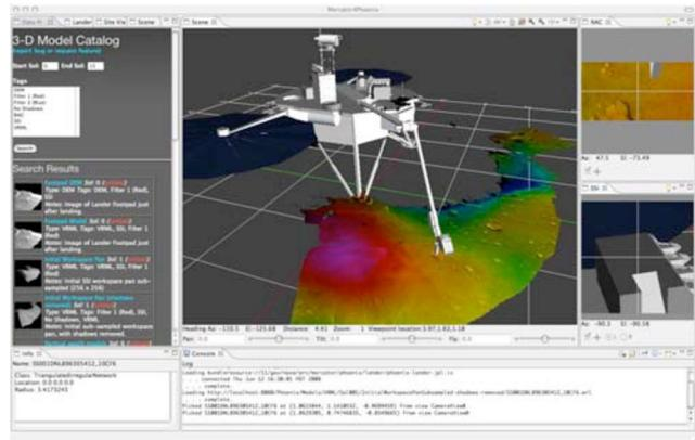
Figure 1. The Mercator 3D visualization environment with simulated Phoenix lander and a terrain model, false color coded by elevation (Lander model credit: NASA/JPL).
