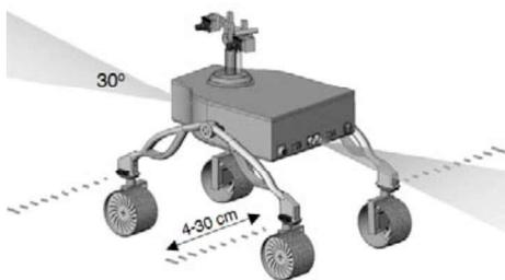
Figure 3. MSTR obstacle detection sensor coverage.
