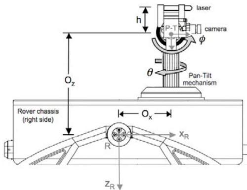
Figure 4. Pointing kinematics.
