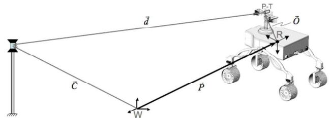
Figure 5. Rover localization geometry.
