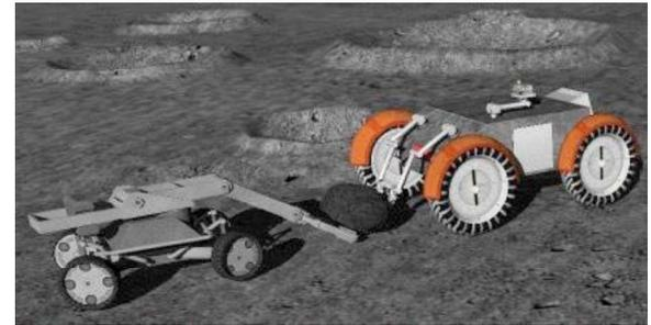
Figure 4. Lunar sample retrieval scenario showing the retrieval rover approaching the nonfunctional rover (top) and start of simplified teleoperated sample retrieval using the robotic arm.
