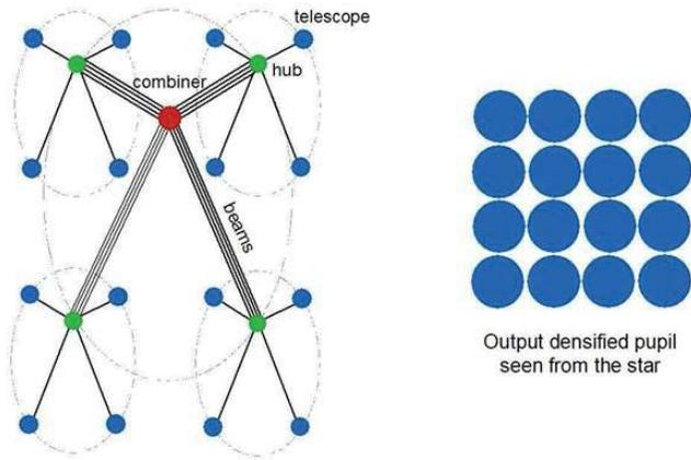
Figure 4. OVLA hypertelescope with 4 rings of 4 telescopes each.
