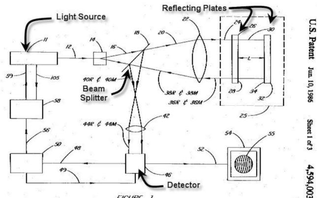
Figure 2. Fizeau interferometric device for measuring wavefronts [1].
