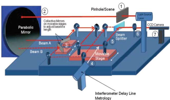
Figure 1. Phase 1 – Macho Mengi Interferometer prototype.
