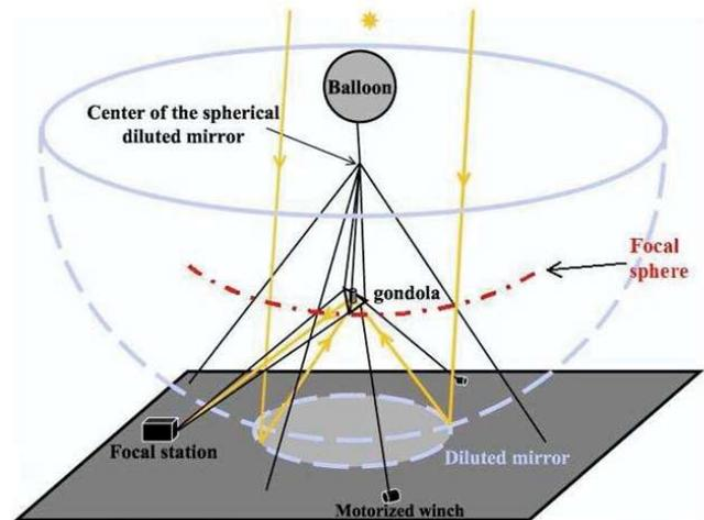
Figure 3. Optical Design of Carlina hypertelescope.
