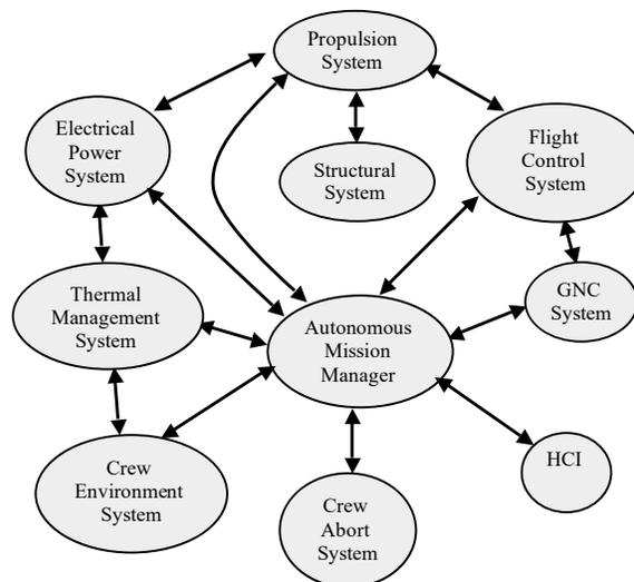
Figure 2. Vehicle systems and autonomous mission management interactions.
