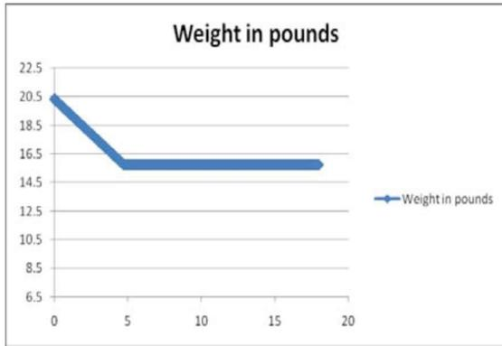
Figure 6. Predicted weight loss of 2008-09 rocket versus time in seconds.
