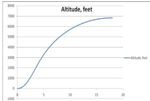
Figure 3. Predicted altitude of 2008-09 rocket versus time in seconds.
