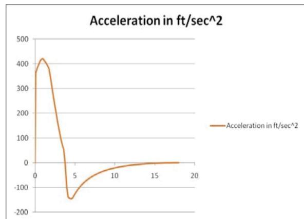
Figure 5. Predicted acceleration of 2008-09 rocket versus time in seconds.
