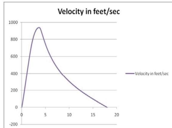
Figure 4. Predicted velocity of 2008-09 rocket versus time in seconds.
