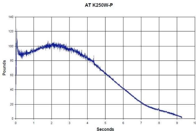
Figure 9. Thrust curve certification for K-250 motor [5].
