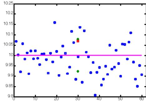
Figure 3. Comparison of  $y^2$  coefficient predicted by inverse method using BPNN output locations to  $y^2$  coefficient predictions by inverse method using randomly chosen locations for the quadratic load function  $f(x, y) = 2x^2 + 10y^2$
