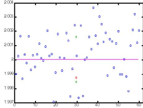
Figure 2. Comparison of  $x^2$  coefficient predicted by inverse method using BPNN output locations to  $x^2$  coefficient predictions by inverse method using randomly chosen locations for the quadratic load function  $f(x, y) = 2x^2 + 10y^2$
