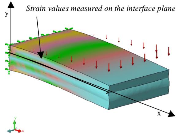
Figure 1. FE model of Transversely Loaded Cantilever Sandwich Structure.
