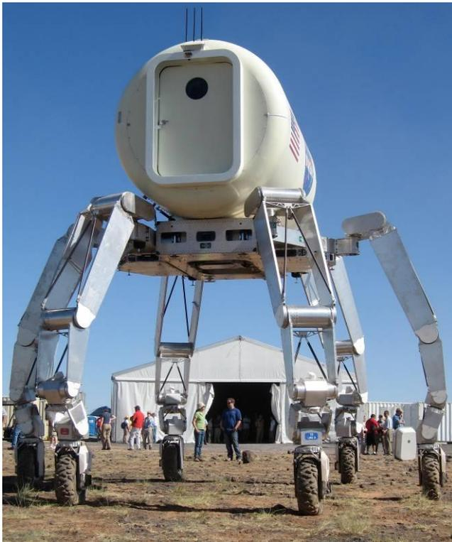
Figure 9. Half-scale ATHLETE robot prototype carrying mockup habitat module
