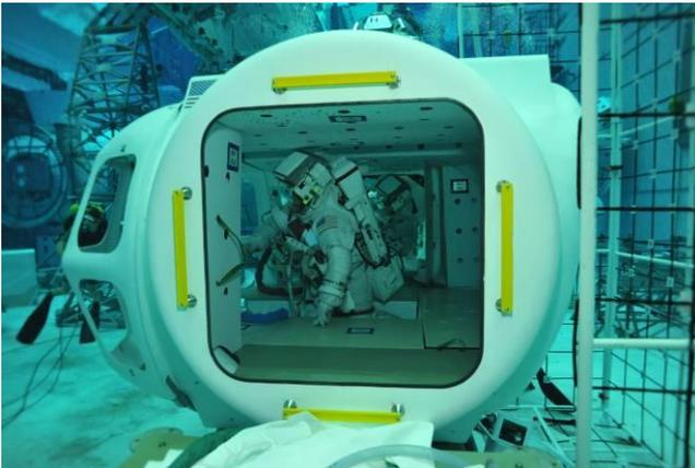
Figure 6. Neutral buoyancy test of ingress/egress for Habitable Airlock configuration
