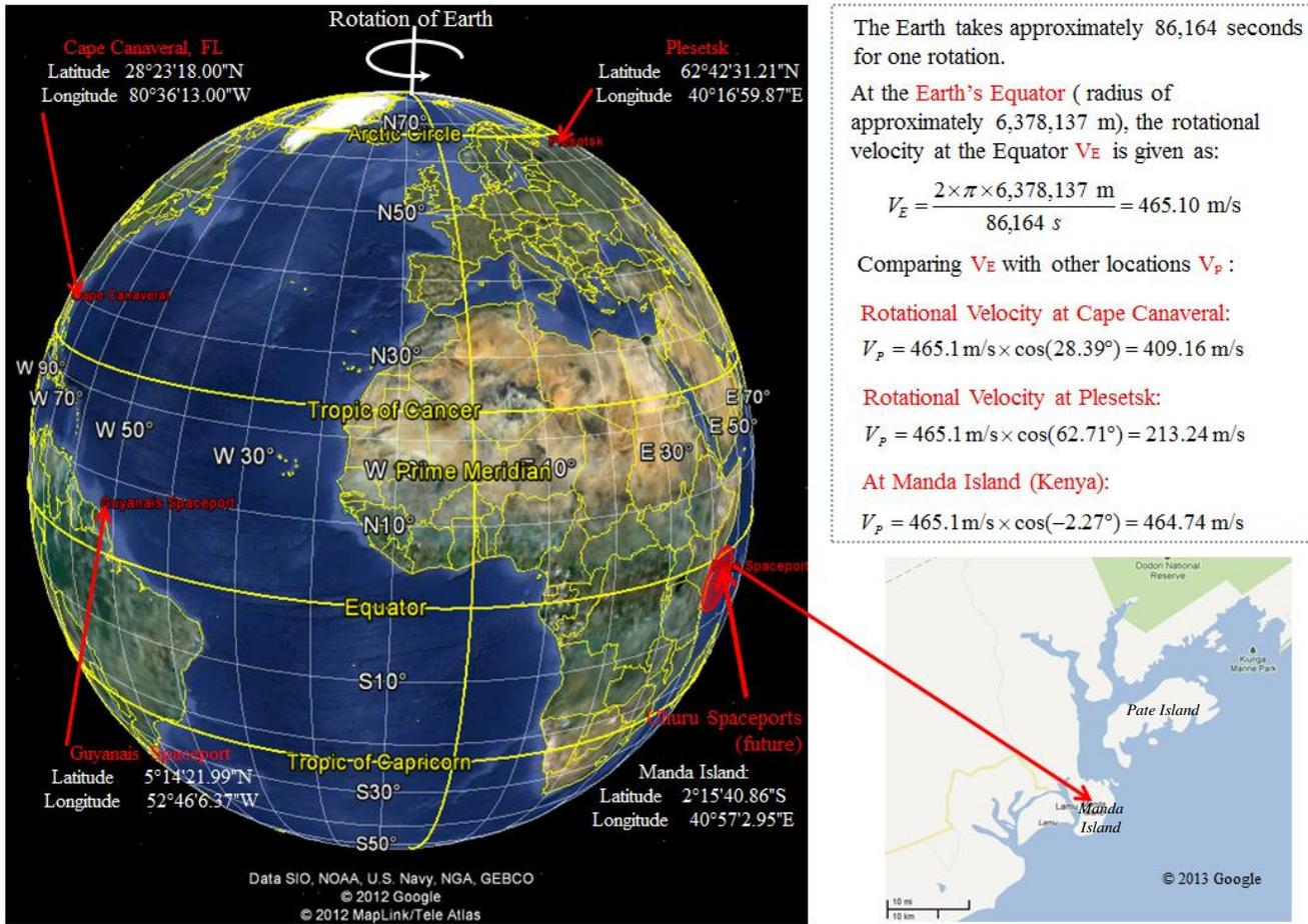
Figure 2. Geo-physical advantages and comparison of Manda Island with other spaceport orbital velocities
