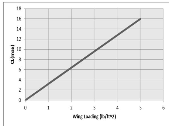
Fig 4- Effect of CL<sub>max</sub> on wing-loading.
