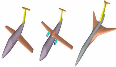
Figure 14. Examples of aircraft configurations that can be analyzed using NeoCASS: a small size trainer (left), a twin engine regional aircraft (middle) and a transonic cruiser (right).
