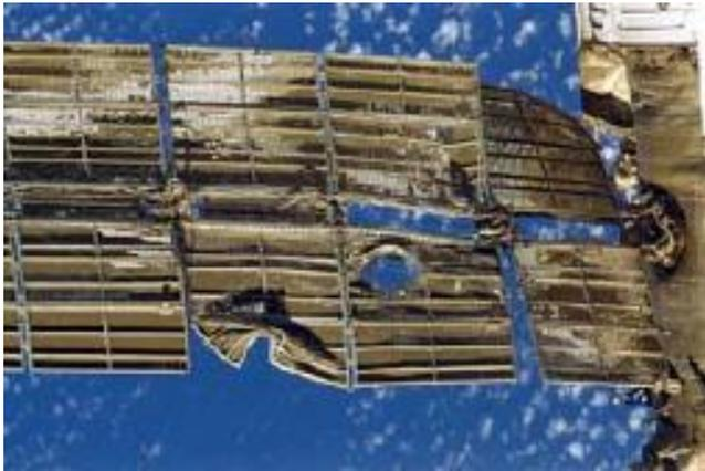
Figure 7. Solar array on Mir Spektr module with damage caused by the Progress collision
