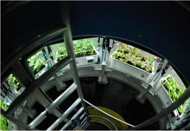
Figure 2. Plant growth chamber inside the Deep Space Habitat mockup at NASA Johnson Space Center
