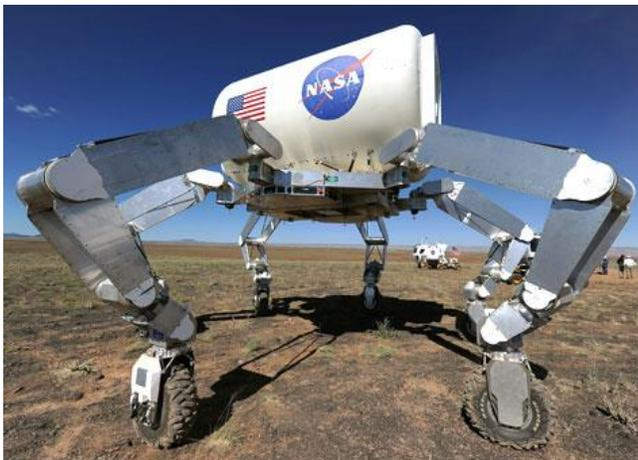
Figure 3. ATHLETE cargo manipulator with SEV pressurized rover in background
