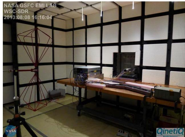
Figure 3: RE02 30 MHz to 200 MHz Vertical Polarity
