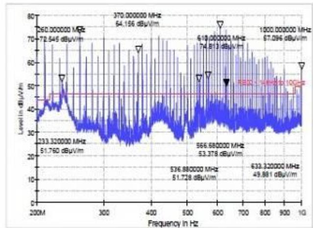
Figure 16: RE02 Test Results 200 MHz to 1 GHz
