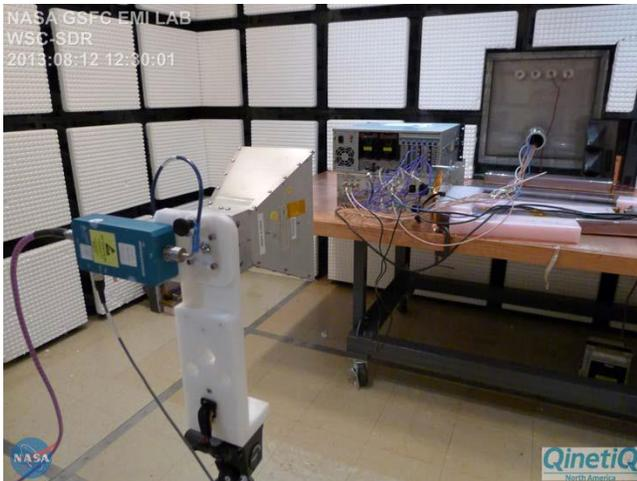
Figure 6: RE02 1 GHz to 10 GHz Horizontal Polarity
