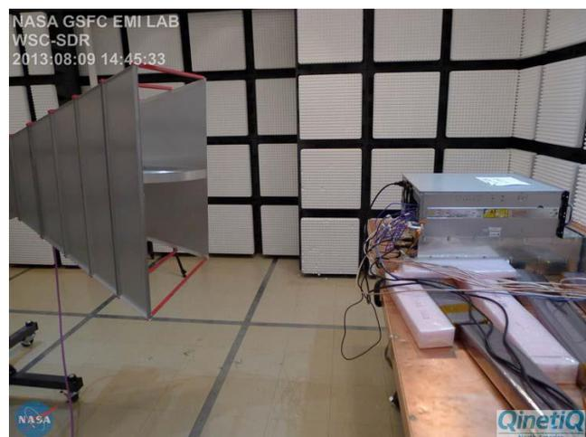
Figure 4: RE02 200 MHz to 1 GHz Horizontal Polarity
