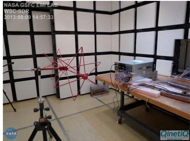
Figure 2: RE02 30 MHz to 200 MHz Horizontal Polarity
