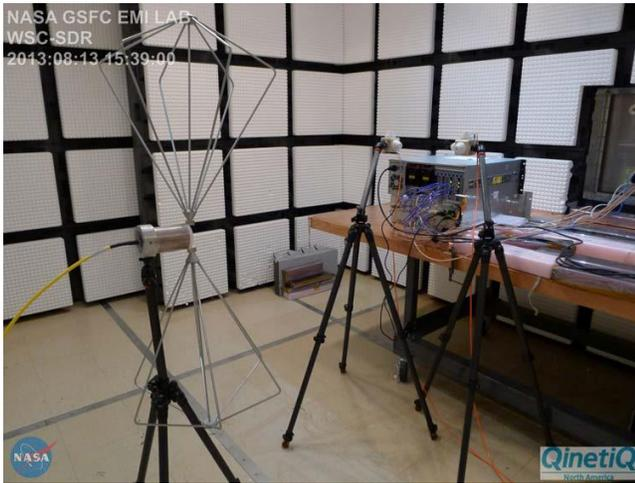
Figure 10: RS03 30 MHz to 200 MHz Vertical Polarity
