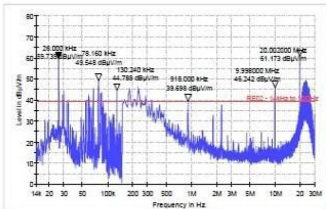
Figure 14: RE02 Test Results 14 kHz to 30 MHz
