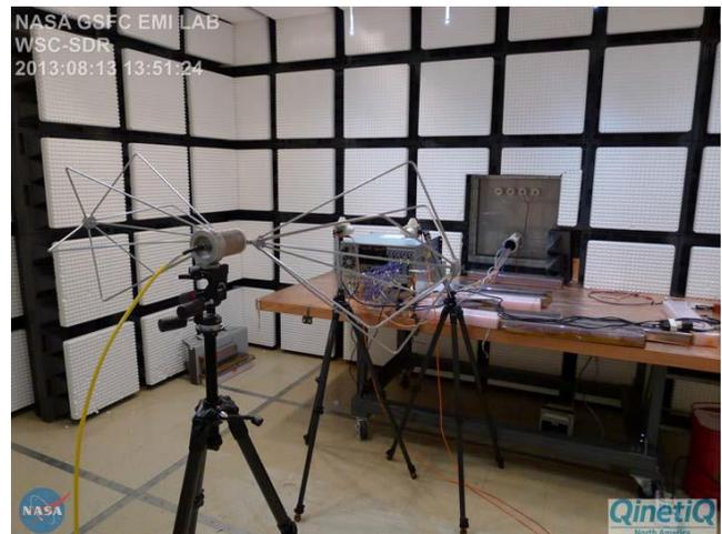
Figure 9: RS03 30 MHz to 200 MHz Horizontal Polarity
