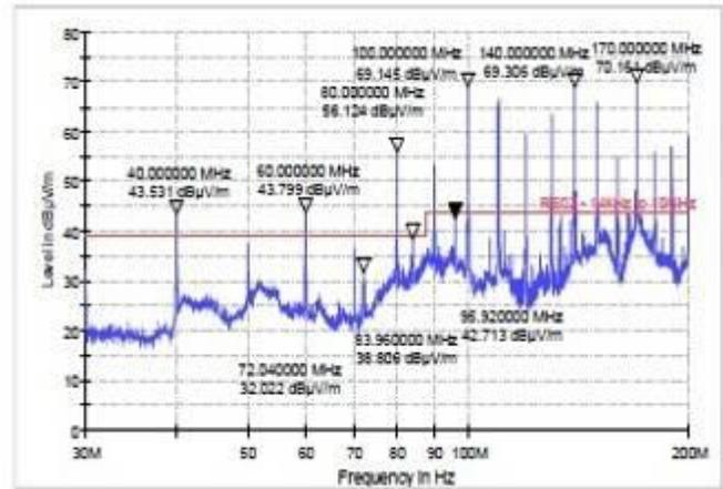
Figure 15: RE02 Test Results 30 MHz to 200 MHz
