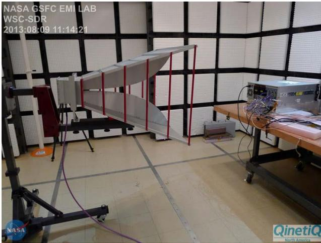
Figure 5: RE02 200 MHz to 1 GHz Vertical Polarity
