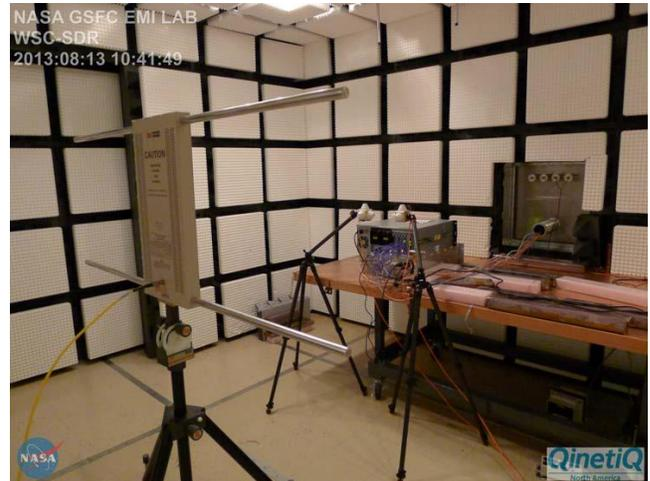
Figure 8: RS03 14 kHz to 30 MHz
