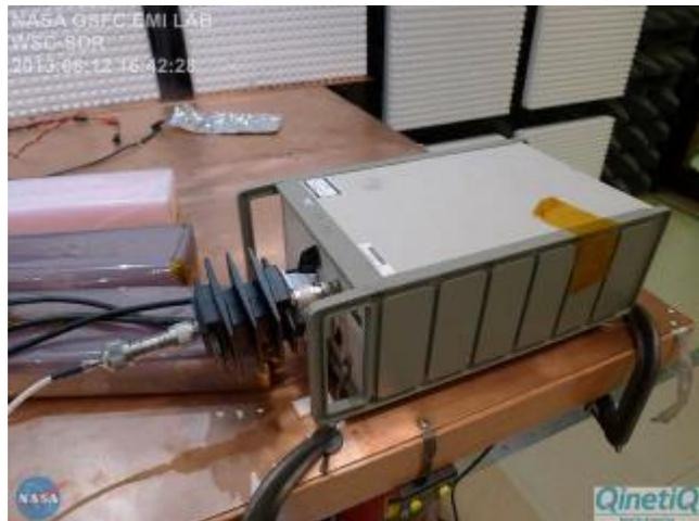
Figure 11: CE03 Equipment Setup
