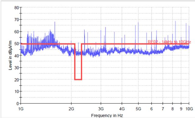
Figure 13: RE02 Test Results 1 GHz to 10 GHz
