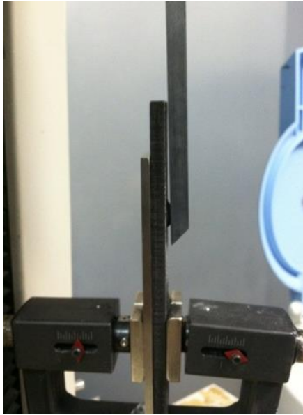
Figure 3. The length of the test specimen allowed a moment arm to be created once the force of the wedge was applied.
