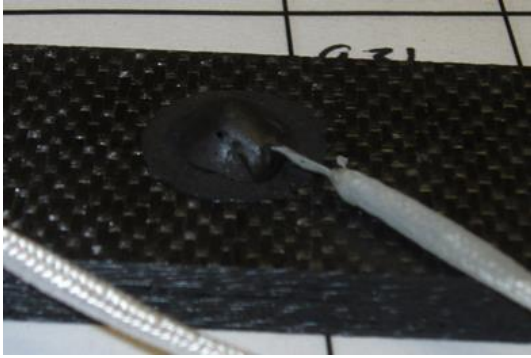
Figure 1. The practice of covering the TC junction and exposed wires was altered to a two part silicone injected into a “button” shaped acrylic mold to be used on test specimens.
