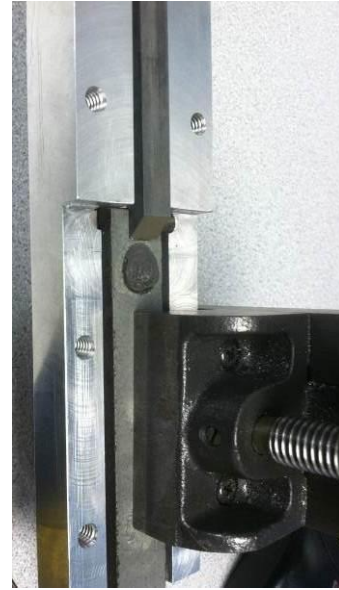
Figure 5. Example specimen clamped into MTS fixture prior to loading.
