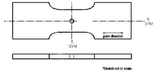
Figure 3 Sample Coupon Specimen
