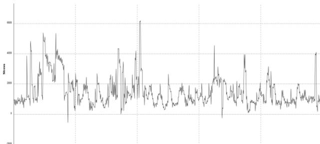
Figure 14 Sample F-16 Block 50 UV1M Un-Truncated Spectrum for a Single Flight
