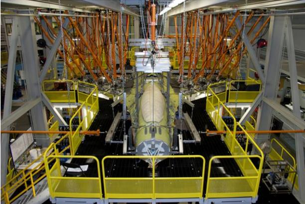
Figure 1 Full Scale Durability Test Aircraft in Fixture
