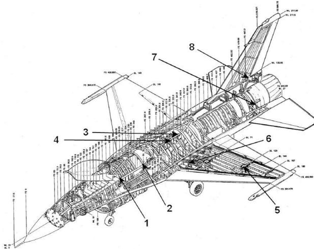
Figure 2 Approximate Locations of the Control Points on F-16 airframe (Corresponds to Table 1 Part Numbers)
