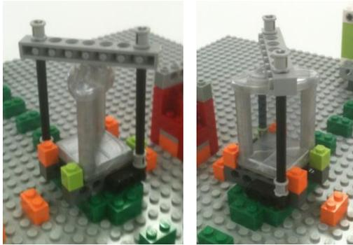
Figure 7: Beam Splitter Mount
