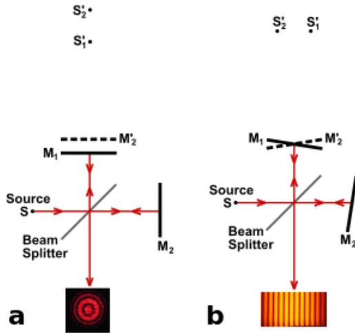
Figure 2: Formation of fringes in a Michelson interferometer [3]
