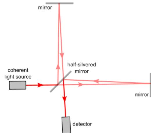
Figure 1: The light path through a Michelson interferometer [2]
