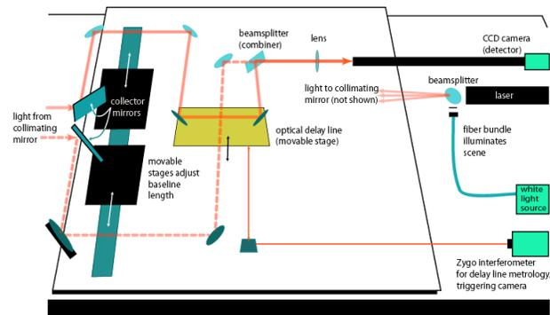
Figure 10: NASA GSFC Wide-Field Interferometer [5]
