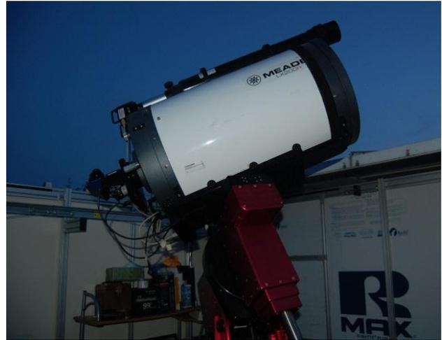
Figure 3: 16" Telescope on Motorized Mount
