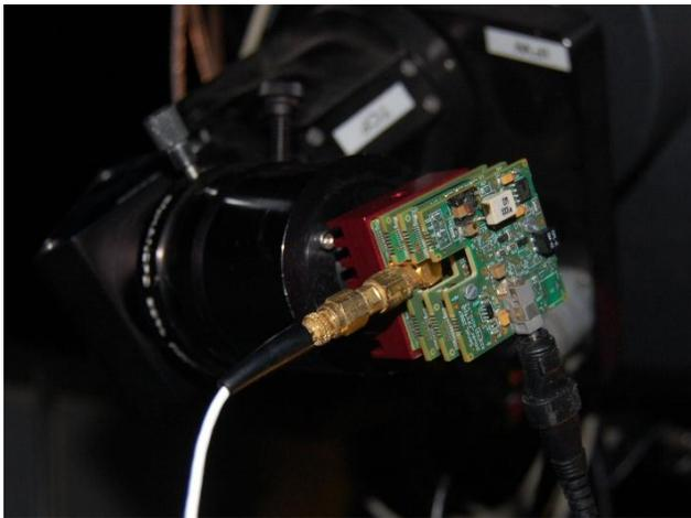
Figure 6: Photon Sensor [SensL APD SPM Mini 1020]
