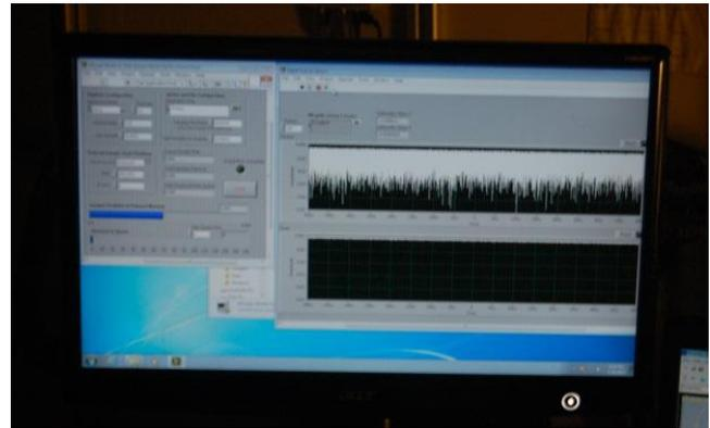
Figure 7: Data Acquisition Screen - Showing Photon Strikes and Intensity on Photon Sensor
