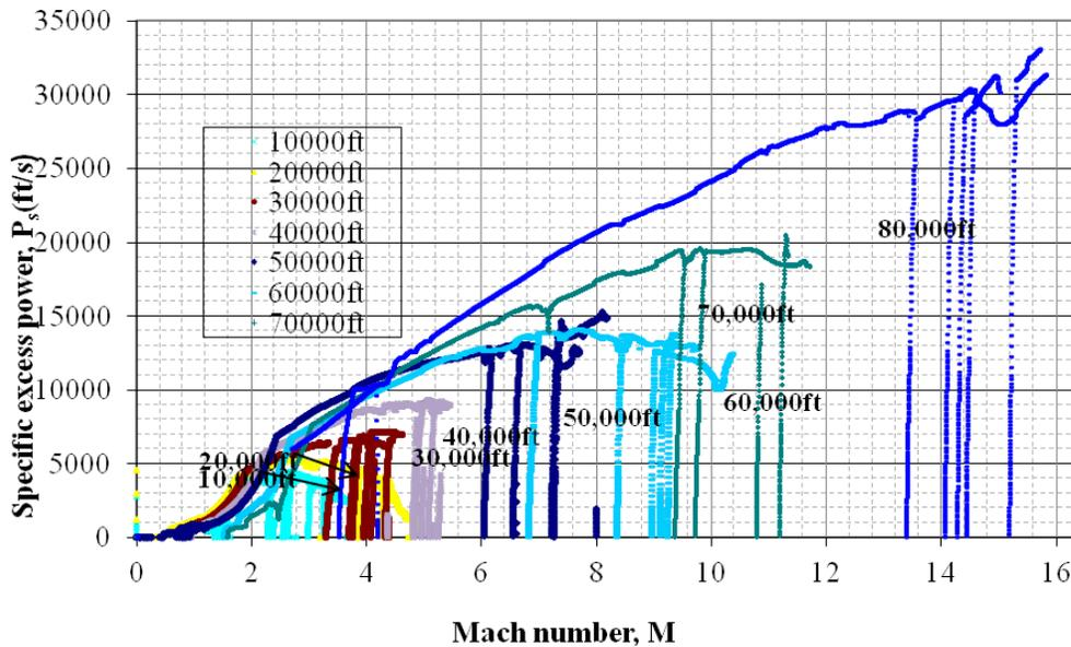
Figure 4. Specific Excess Power,  $P_s$  (ft/s) versus Mach number,  $M$  for X-30 aircraft. (Direct  $P_s$  calculated by display)
