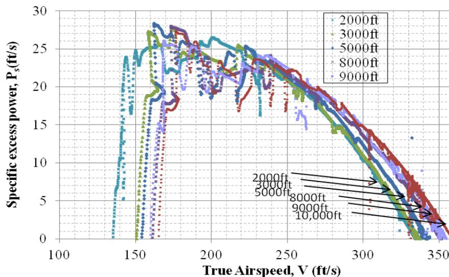
Figure 3. Specific Excess Power,  $P_s$ (ft/s) versus True Airspeed,  $V$  (ft/s) (Direct  $P_s$  calculated by display)
