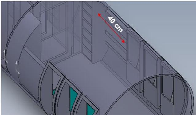
Figure 2. Length Available for Stowed Maintenance Workstation
