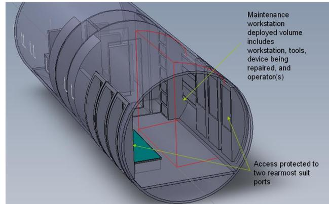
Figure 4. Deployed Workstation Volume Envelope
