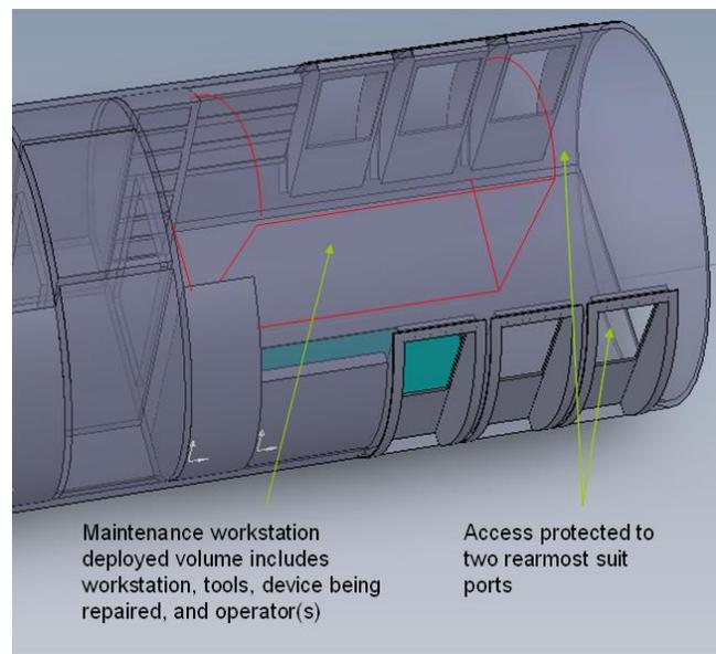
Figure 5. Protected Access to Two Suit Ports for EVA
