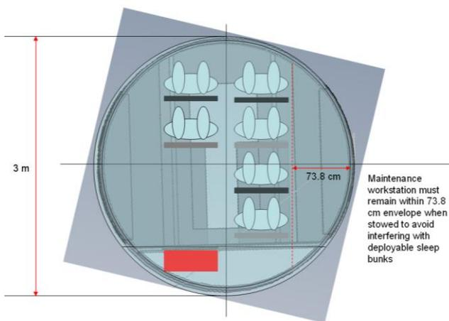
Figure 3. Crew Bunks Clearance for Stowed Maintenance Workstation
