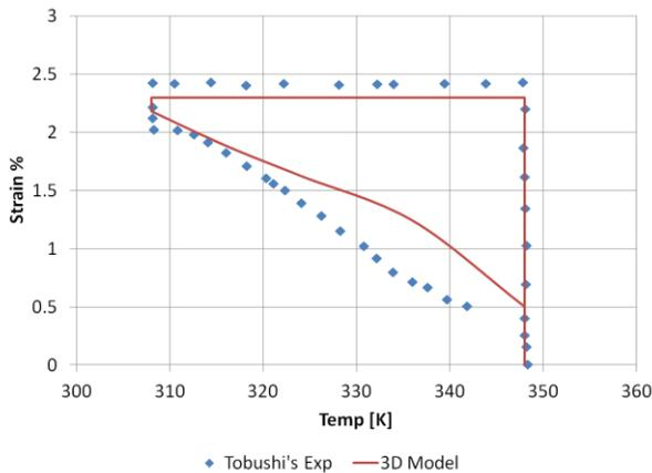
Figure 6. Strain vs. Temperature model validation
