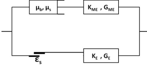
Figure 3. Modified Maxwell-Zener Model incorporating Tobushi's slip element.
