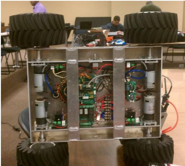
Figure 4. Robot Electrical Subsystem
