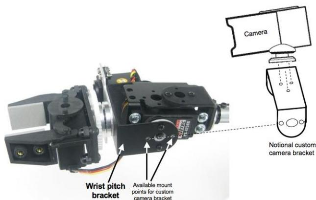
Figure y. Available screw holes on the wrist pitch bracket for one custom camera bracket mounting option, and a corresponding notional bracket design.
