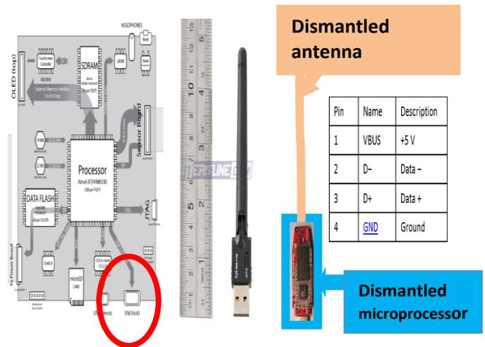
Figure 8: Wi-Fi component Breakdown
