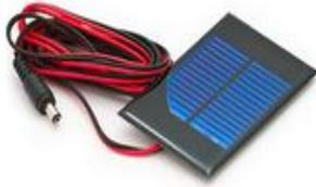
Figure 9: Sparkfun Solar Cell[3]
