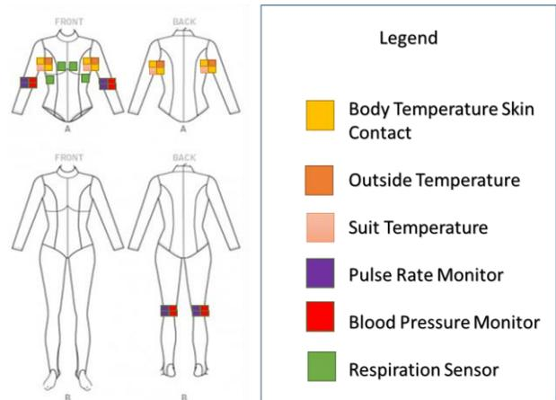
Figure 8: Placement of sensors on NSBE MDRS suits
