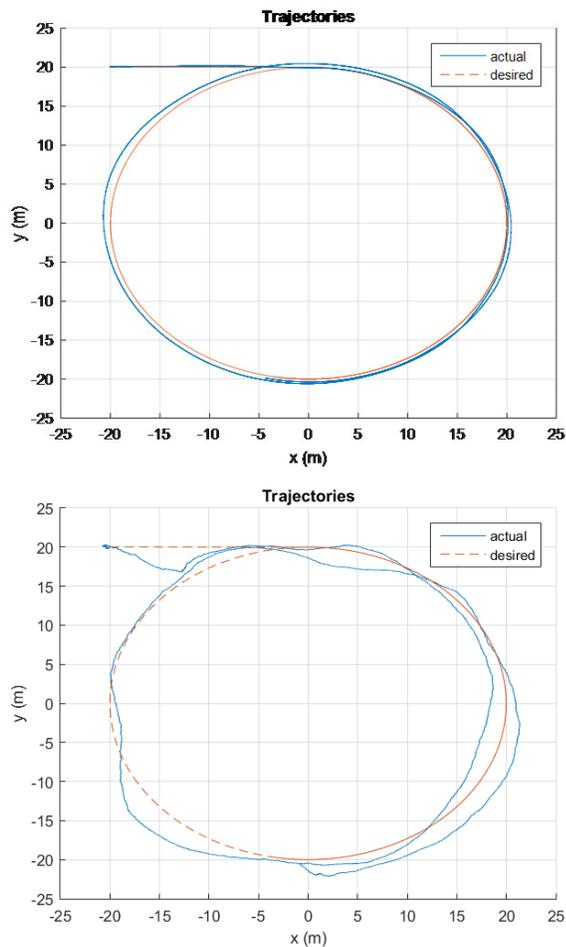
Figure 5: Trajectory under a disturbance with a SNR of 100 dB (top) and 80dB (bottom).
