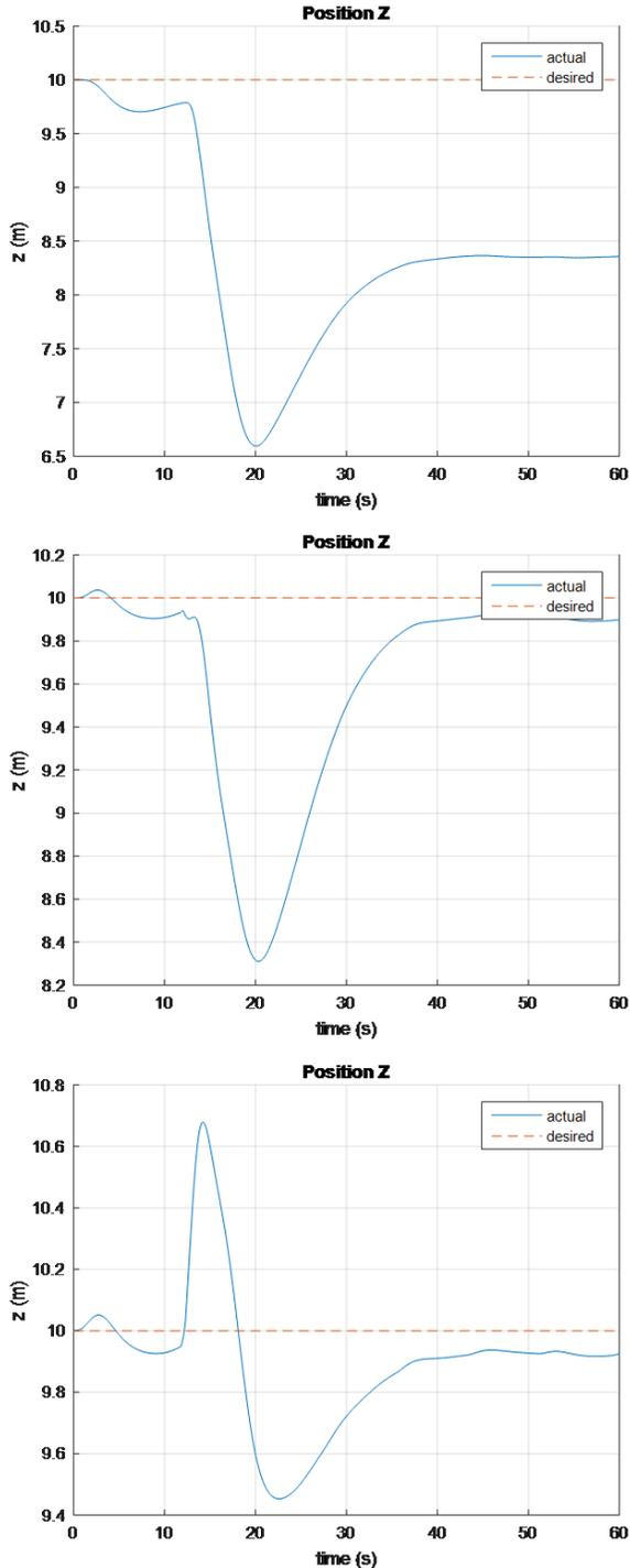
Figure 4: Z position of lander using linear control (top) simple geometric control (middle) and weighted geometric control (bottom).
