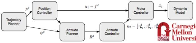
Figure 2: The Cascade PD control hierarchy.
