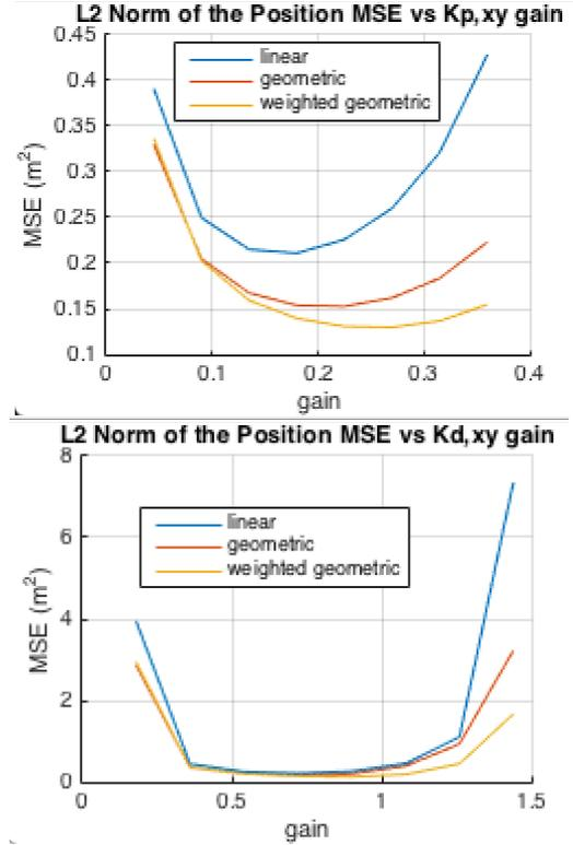
Figure 3: Mean squared position error under a range of  $K_{p,x}$  (top) and  $K_{d,x}$  (bottom) gains, per controller.
